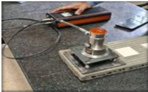
Mobile Pull-off tester
