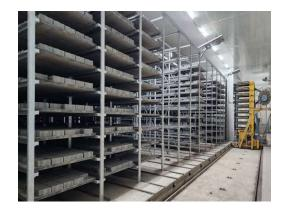
Curing of blocks take place in controlled conditions in enclosed chambers
