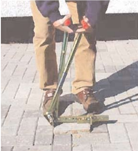
Special block removal/extractor tool
