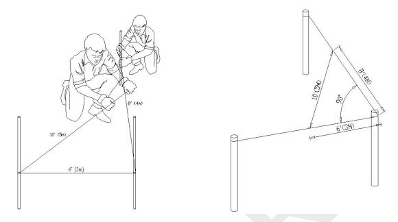
A quick way to establish a line perpendicular to an edge (no corner walls) is with the following procedure:
