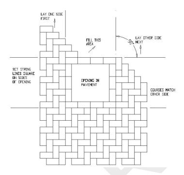
Plan your installation to begin along a straight line and preferably in a corner which is easily accessible. Make absolutely certain that the beginning corner is a true 90 degree angle. If the intersection of 2 sides is not a true 90 degree angle, you must establish a 90 degree starting point.
